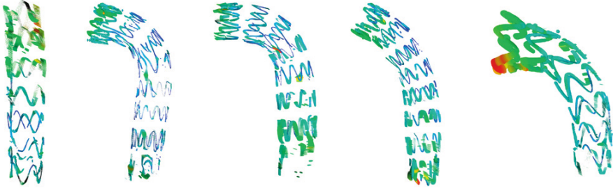
Figure 2.18: Global deformation (color-coded) for a few stent grafts. (Image courtesy of G. Langs from [75].)
